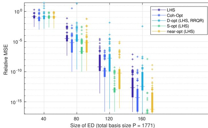
Figure 1: Surrogating the Ishigami function with sparse PCE: Plot of relative MSE against number of design points for different ED sampling techniques (sparse solver: LAR, basis: total degree  $\leq 20$ , 100 replications).
